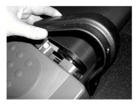
2. With flat blade screwdriver, remove Grommet and Washer, discard old washer and re-install the grommet. Use caution to prevent injury or damage to paint.
